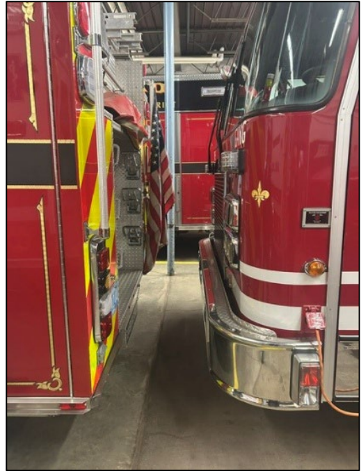
Very Limited Clearance Between Apparatus in the Bays
